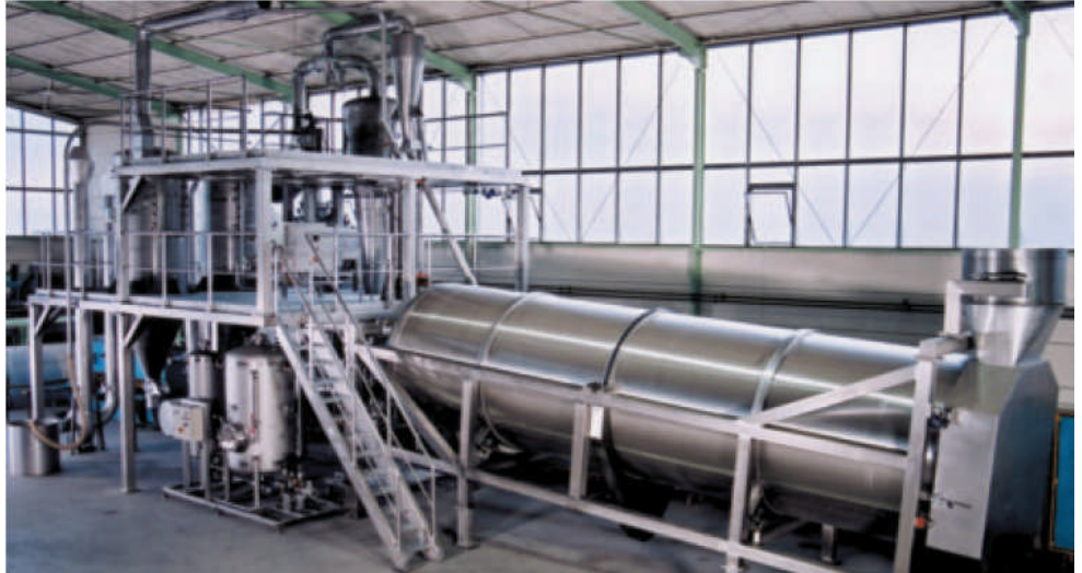
Fig. 9: Production-line view of a CEREX standard puffing system, ready for installation in a production plant.
