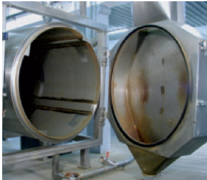
Fig. 8: Expansion conduit with open door.
